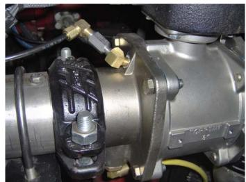
wire tied to a convenient location that will allow easy access for maintenance. The zerk fitting that comes standard on the Torrent SVS valve can be removed from the valve and reused by attaching it to the bulkhead. This fitting has a seal inside; do not substitute an automotive grease fitting.
