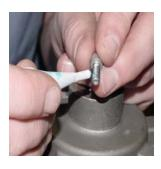
STEP 1 Apply Loctite No. 242 p/n: 029-0010-01-0 to mounting screw threads p/n: 018-1004-93-0 prior to installation as shown.
