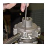
STEP 2 Install mounting screw (p/n: 018-1004-93-0) as shown.
