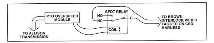
The module can power a relay with a normally closed contact. By adjusting the overspeed module to a speed just above idle, the relay will energize, opening the interlock whenever the engine is above idle speed.
