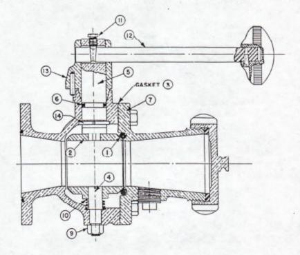
LUBRICATION Using a brush, lubricate the face of the ball (2) with a waterproof grease once a week. Additionally, on a suction valve, squirt some oil in the space next to the rubber washer to lubricate the swivel balls. The remote control linkage connecting the valves should be lubricated monthly.
