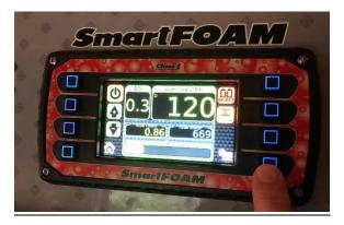
3. The menu screen should be showing. Push the top right button next to the Calibration/Configuration symbol on the screen.
