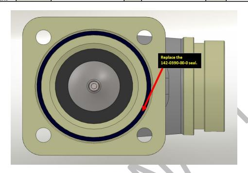
Conclude this replacement by remounting the intake relief valve on the pump, repeating this procedure on any other desired intake relief valves on the pump, and lastly conducting a standard pump air leak test.
