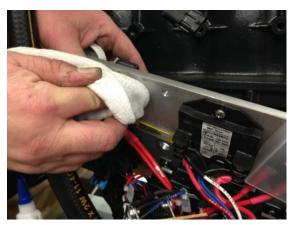
8. Apply 1.5" long strip of VHB double sided tape to relay between mounting holes as shown. Press on firmly.
