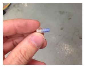
10. Insert screw from rear of panel into bottom mounting hole as shown, and thread into relay housing 1-2 threads.
