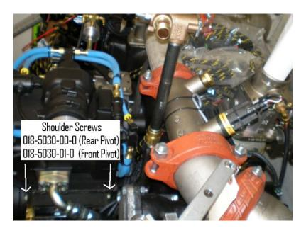
The following procedures are provided for replacement of the Compressor Belt Adjustment hardware. Refer to the illustrations to identify components. (NOTE: Front, Rear, Left and Right are identified from the driver's perspective)
