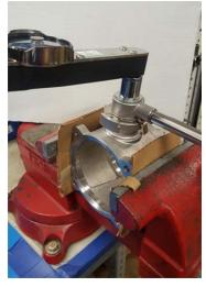
If a valve is found to be moving during pump test, add shim, or replace existing shim with a thicker shim to attain 23 ft-lb of resistance. Check the actuation torque with the ball removed to ensure the locking force is 23 ft-lb (31 n-m) or greater as shown above.
