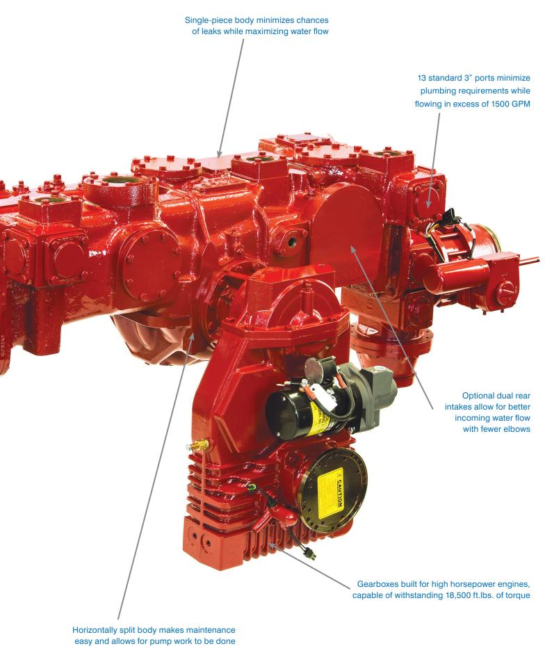
easy and allows for pump work to be done without disturbing plumbing
