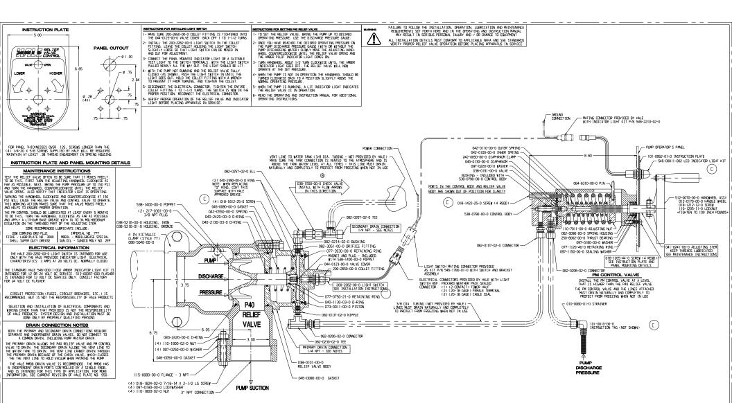
HALE TYPE P40 RELIEF VALVE WITH PM CONTROL VALVE
