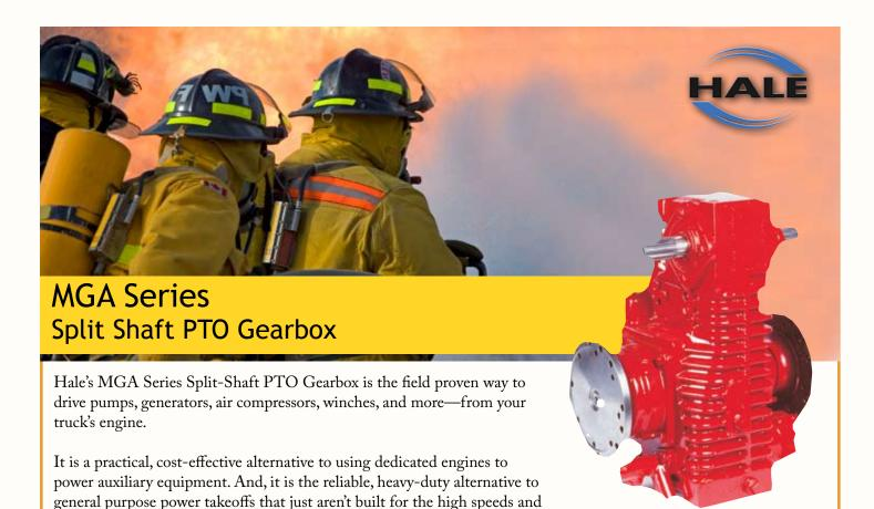
Installed in a midship position between the two halves of a split driveshaft, the Model MGA uses a sliding gear to shift power between the vehicle's wheels and its own output shaft. The sliding gear is positioned by a manual, air, or vacuum powered shift mechanism.
