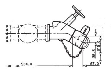
**Dual Flow valve is similar to UK** type but includes capability to lift valve flap for draining hoses
