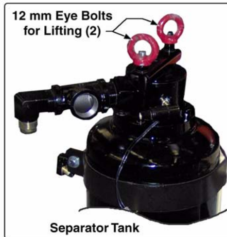
Figure A-4: Lifting Separator Tank
