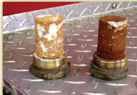
Example of sacrificial corroded anodes
